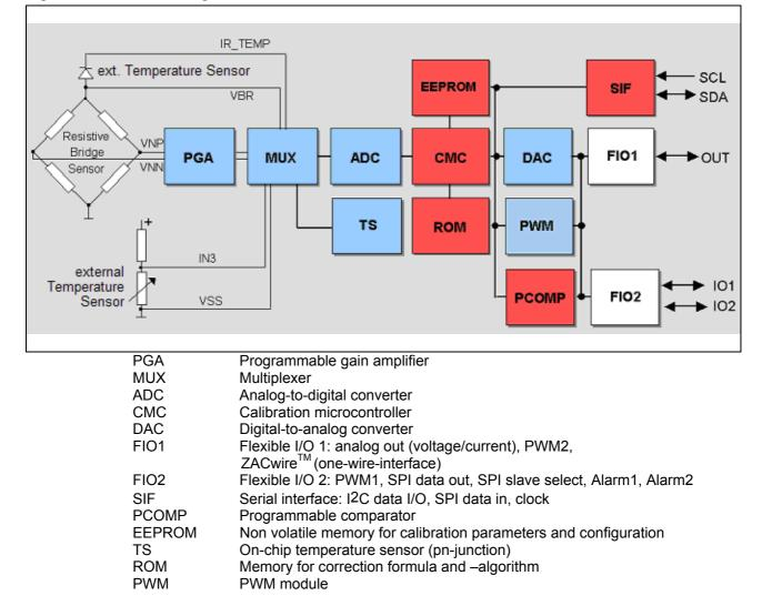
Figure 2.1 Block Diagram of the ZMD31050
